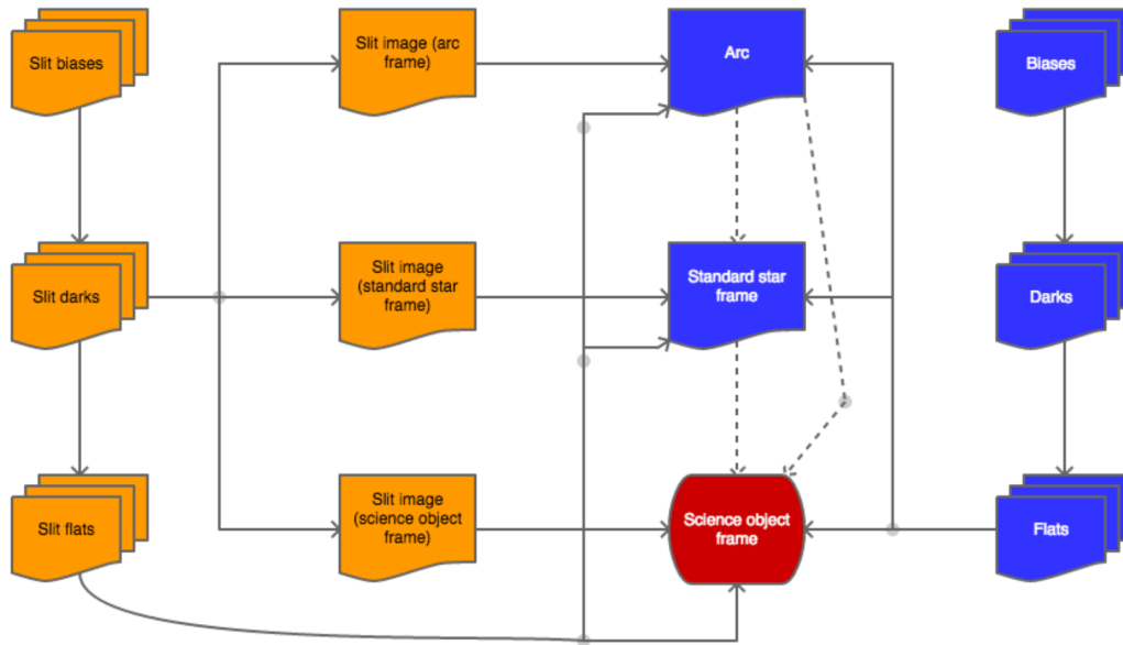
Figure 2.6: GHOSTDR processing flowchart managed by dedicated recipes for each image type. Slit viewer camera images are noted in orange, calibration frames are identified in blue and science frames are shown in red. Solid arrows show required data processing steps that use each of the identified images, whereas the dashed arrows show optional data processing steps that use GHOSTDR data products rather than raw or processed images. Source: Farrell et al. (2022) .
