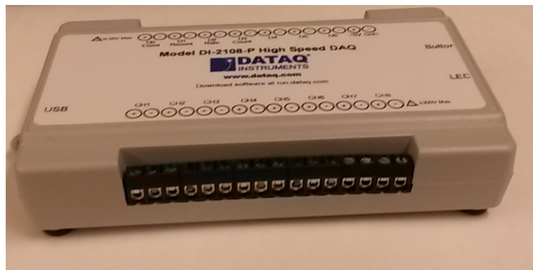
Figure 5.6: Voltage monitor used in Phase 2 [19].
