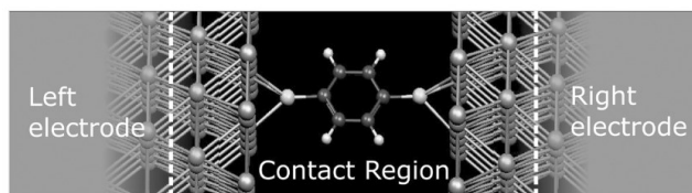
Figure 4.2: Schematic of a device setup for calculation charge transport using NEGF principles.
