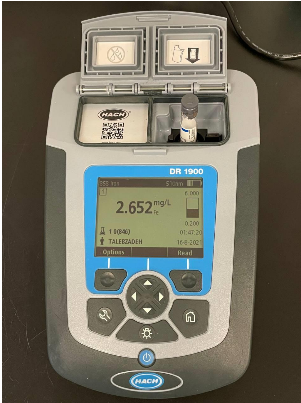
Picture6. Analyzed sample to evaluate the concentration of iron in CWW
