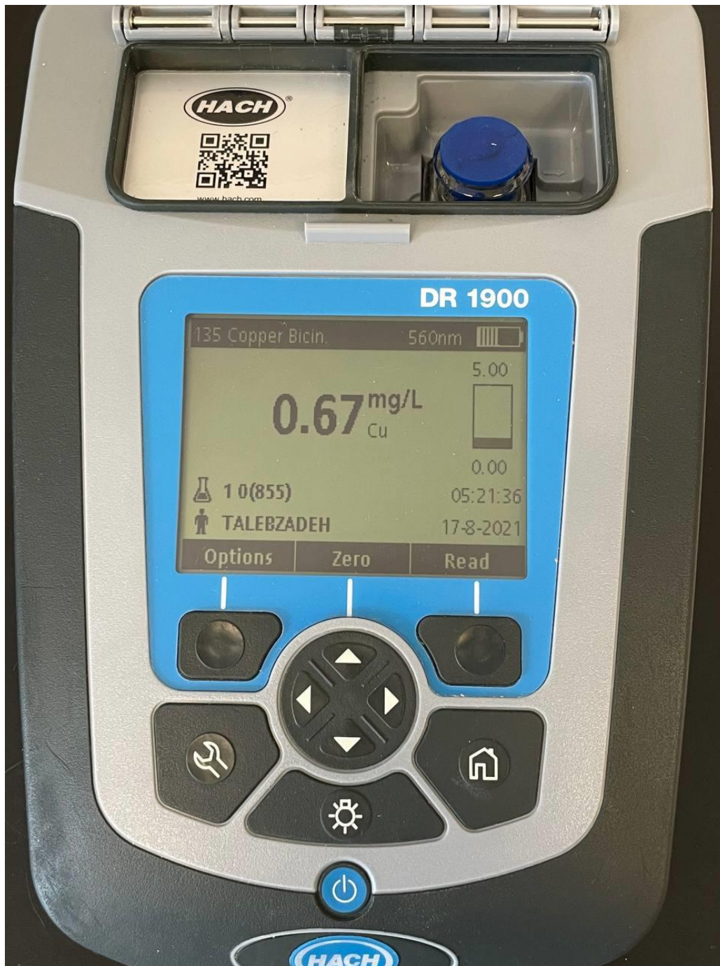
Picture8. Analyzed sample to evaluate the concentration of copper in CWW
