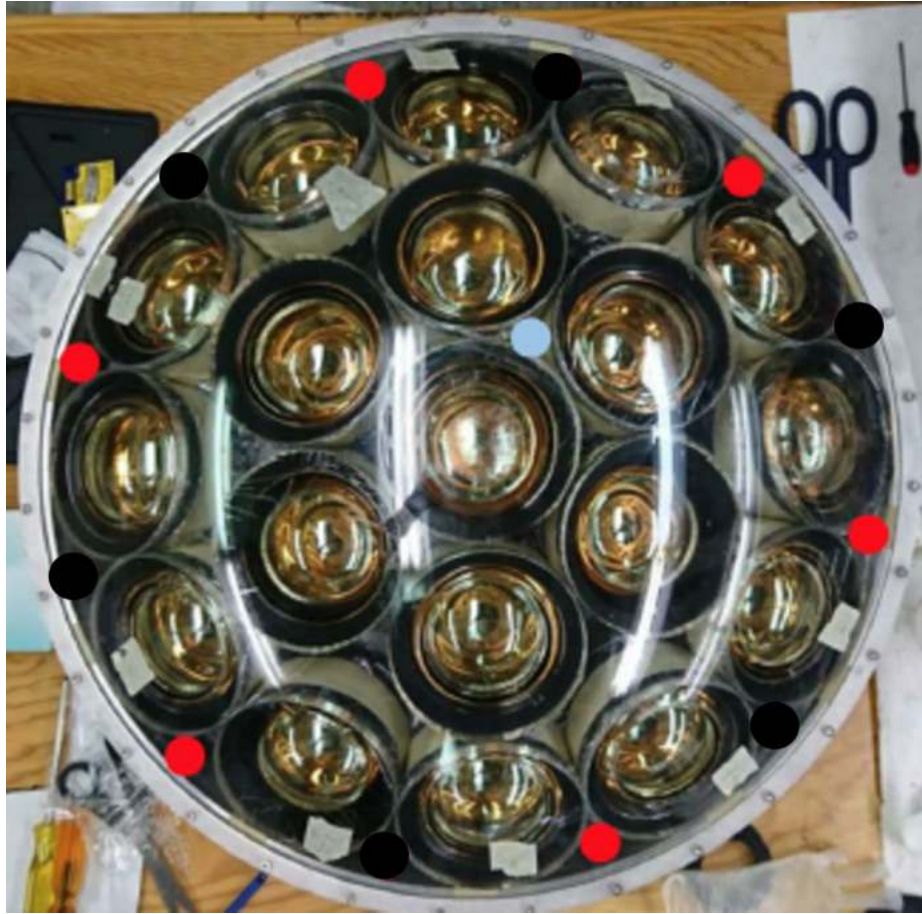
Figure 2.3: Birdseye View of multiPhotomultiplier Tube. Red dots denote planned beacon light pipes, Black dots denote omitted light pipes, Grey dot denotes pulsed light pipe.
