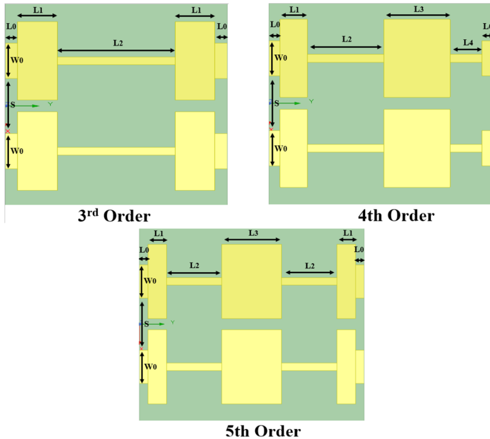
Figure 5.1: Geometrical layouts of third-, fourth-, and fifth-order THz Butterworth filters based on stepped-impedance transmission lines.
