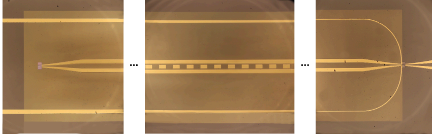
Figure 1.2: Microscopic image of the THz band-stop periodic filter
