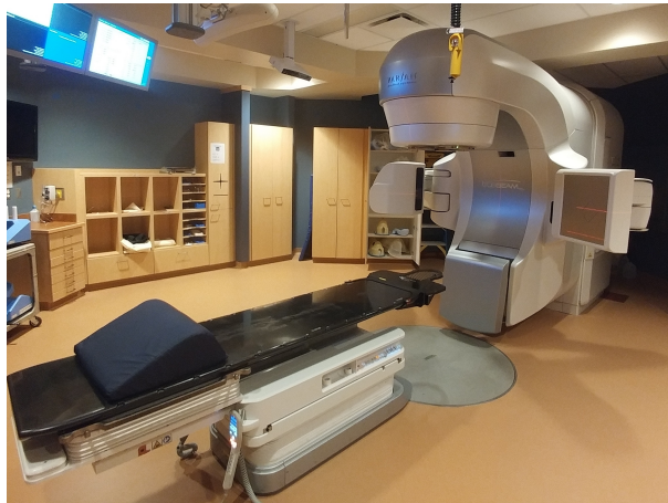
Figure 1.1: Varian TrueBeam STx linear accelerator at BC Cancer - Victoria with gantry and patient couch used for external beam radiotherapy treatment.
