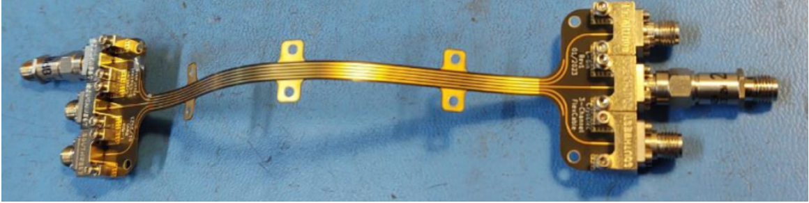
Figure 4.12: Prototype flexline for the 850 GHz module by CryoElec. 46 From the initial analysis of the crosstalk within the flexline in the range of interest for the readout (max 1.3 GHz), the majority of the measured channel isolation was greater than -25 dB.
