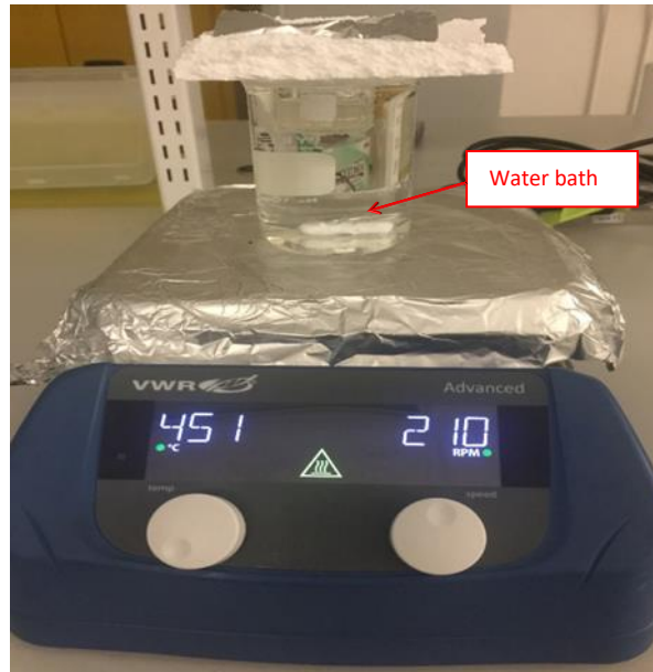
Figure 28: Dissolution process of agarose powder in TBE buffer illustrated within a water bath setup.
