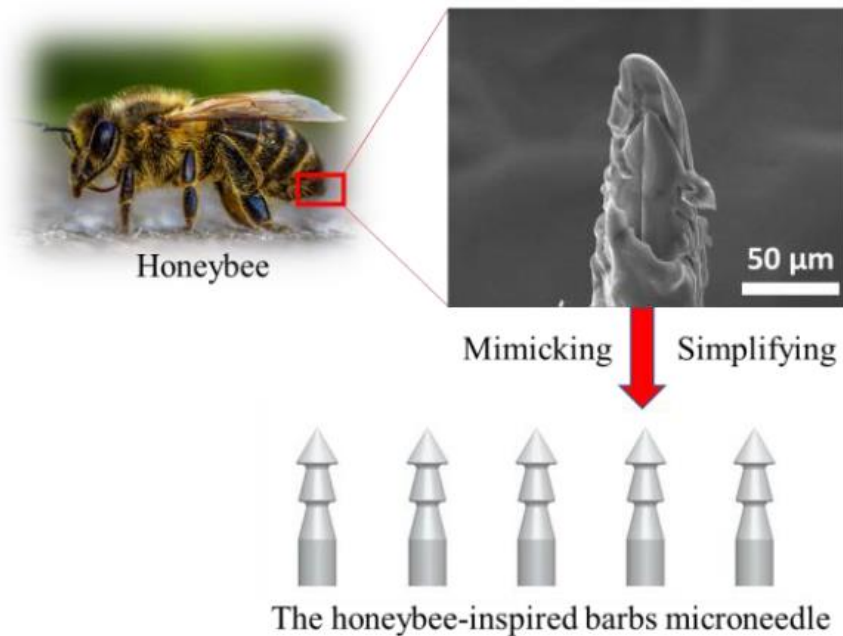
Figure 3: Schematic design of a barbed MN inspired by the honeybee stinger, engineered for easy skin penetration and secure interlocking. [32]
