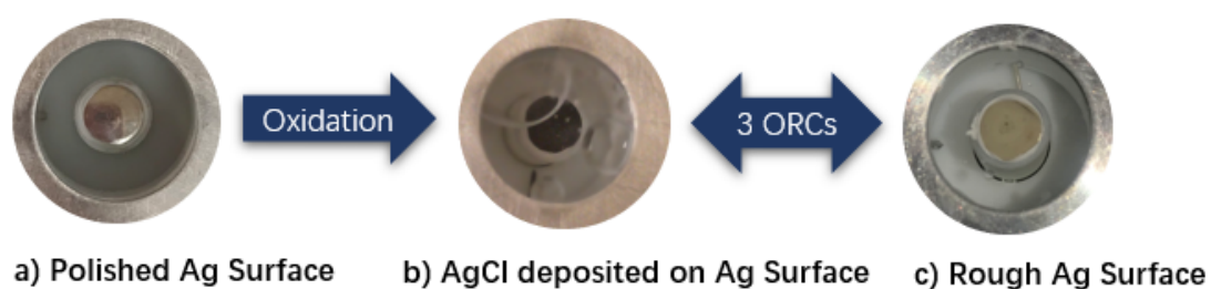
Figure 2.4 Surface appearance when oxidation-reduction cycles (ORCs) are applied during the activation procedure.
