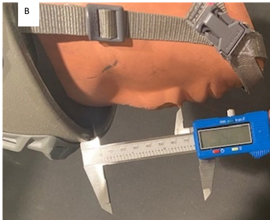
Figure 11: A) Placement of a military helmet onto the Hybrid III headform with correct placement between the nose and helmet brim per the HPI for a military helmet test. B) measurement of the 74mm between the nose and the helmet brim to achieve the correct HPI.
