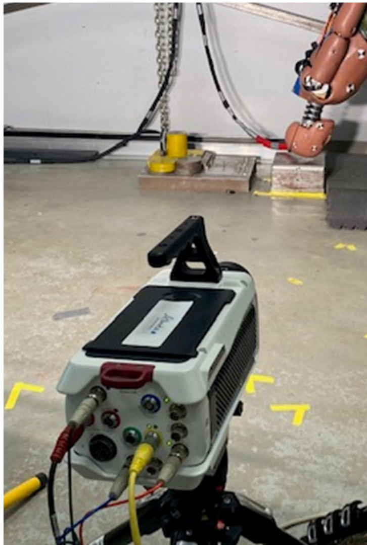
Figure 12: Placement of high-speed camera for full-body impacts to allow for measurement of angle and velocity at impact.
