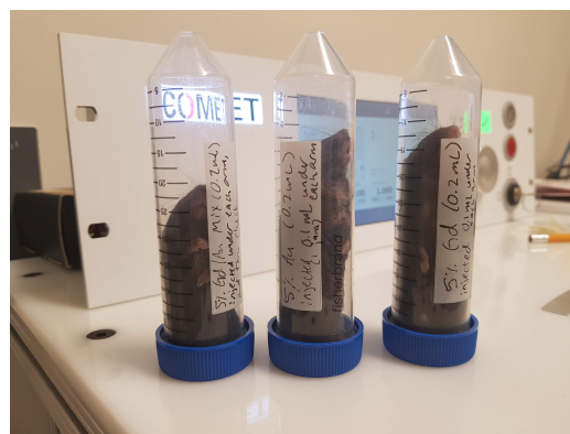
(b) Three contrast-filled mice of mass 20 g, 26 g, and 32 g from left to right.
