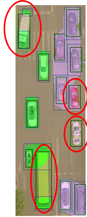
(b) Detection Results: Blue Boxes are the motion detection; Black boxes are the annotation boxes. The circles highlight instances of missed detection
