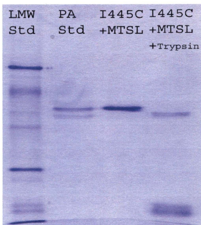
Figure 5.13: SDS-Page gel of 1.66 \mu M 445C PA + MTSL with and without trypsin added, LMW Std included 97.4, 66.2, 45.0, 31.0, 21.5, and 14.4 kDa proteins 32 , the bottom of the 445C PA + MTSL + trypsin lane has a blue band at the bottom of the gel that denotes the presence of trypsin.
