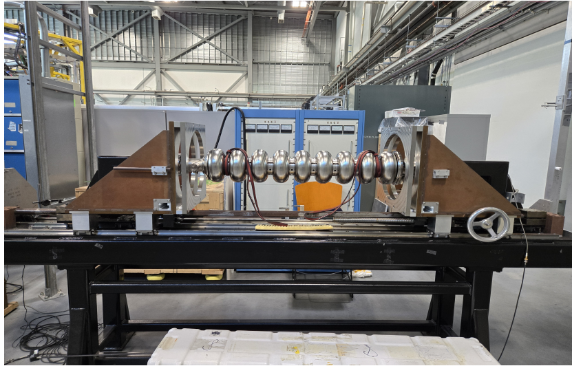
Figure 3.5: The beadpull station used for RF measurements. Attached is the 9-cell 1.3 GHz elliptical cavities used in the plasma processing tests.
