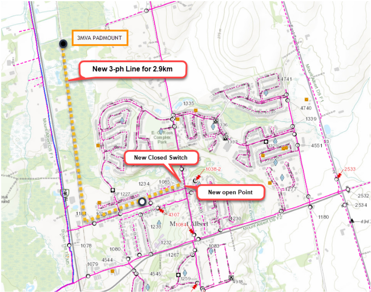
Figure 2.22: Installation location of two 3MVA pad-mount transformers in Scenario 2.
