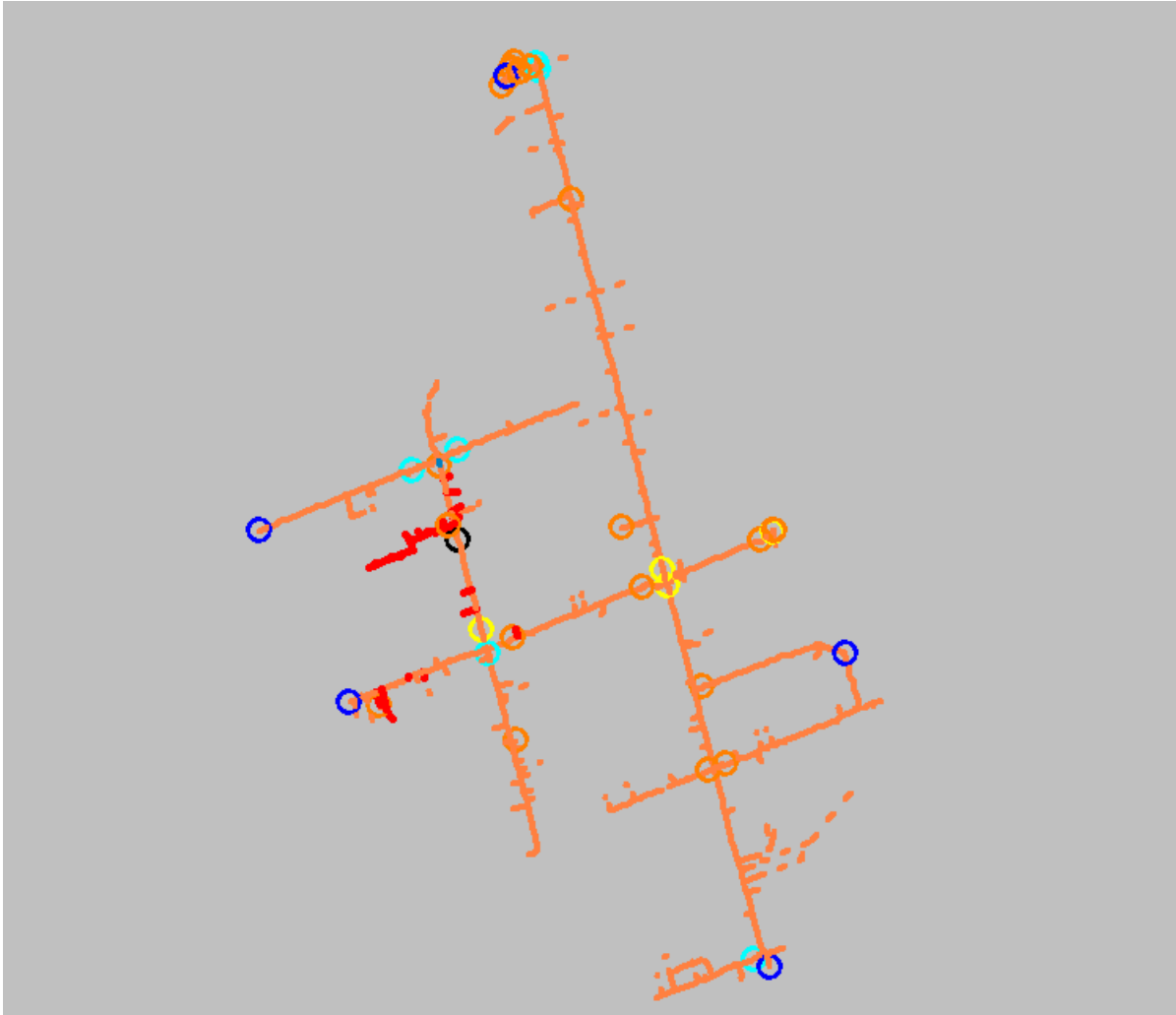
Figure 2.15: CYME results showing the voltage levels for Mount Albert DS: Feeder F3.
