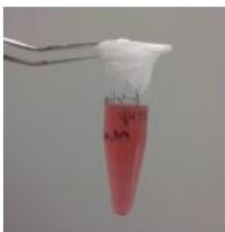
Figure 2. 9 Solution of 1, 9-nonanedithiol and colloidal gold particles with N_{\text{molecule}}: N_{\text{particle}} of 1:1 after incubating for 24 hours.
