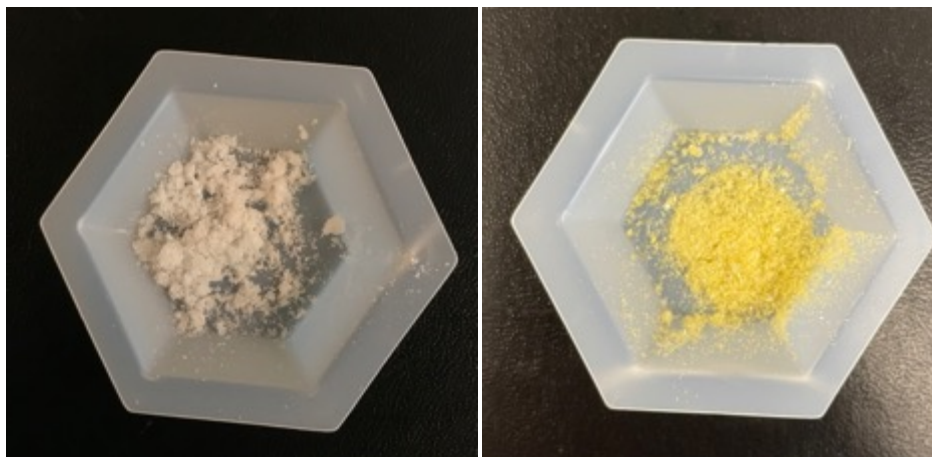
Figure 2.4: Photographs of polyphosphinoborane 2.3a made by deprotonation of 2.1a (left) and polyphosphinoborane 2.3a made by \text{Cp}(\text{CO})_2\text{FeOTf} -catalyzed dehydropolymerization of 2.1a (1 mol%, toluene, 100 °C, 24 h) 11 and discoloured by residual iron species (right). Photographs taken by Matthew A. Wiebe.
