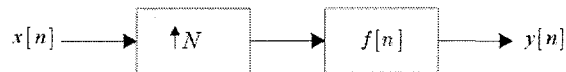
Figure 11. N -fold upsampler followed by an anti-imaging filter with impulse response f[n] .
