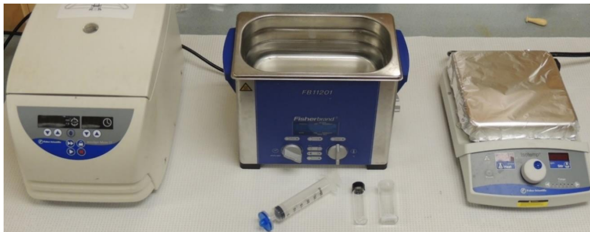
Figure B-SI-1 Only simple labware is required for the synthesis of the nanoshells. Left to right: Microcentrifuge, ultrasonic bath, 0.22 \mu\text{m} syringe filter, vials, stir bars and stirring plate.
