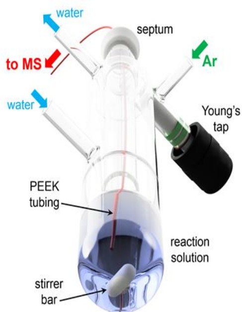
Figure 1.12. Representation of a pressurized sample infusion (PSI) customized flask.
