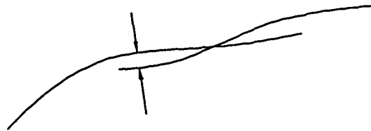
shift between global/partial model curves due to imaging registration errors
