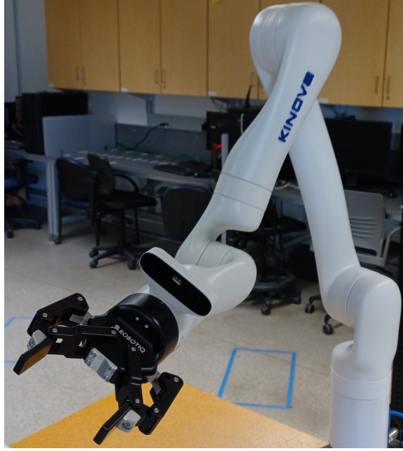
Figure 5.4: The physical experiment setup including the Kinova® Gen3 robot and the Robotiq® 2F-85 gripper
