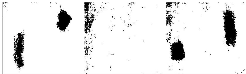
Figure 26: IRT- Area accuracy computation:100 mm slab using MATLAB Software
