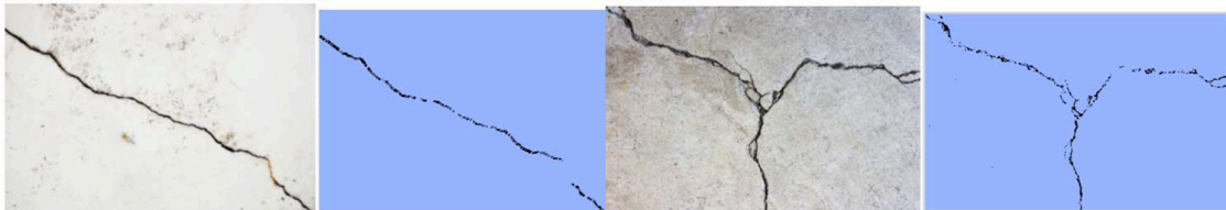
Figure 4: HSV thresholding crack output
