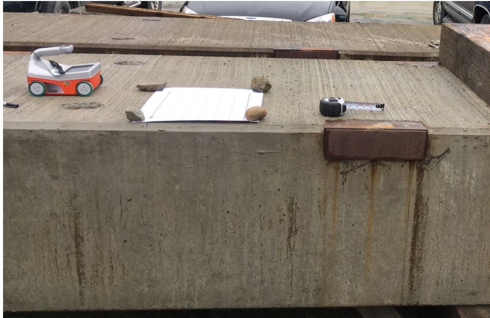
Figure 35: GPR and Profoscope tests on the top the precast girder at Surespan Structures
