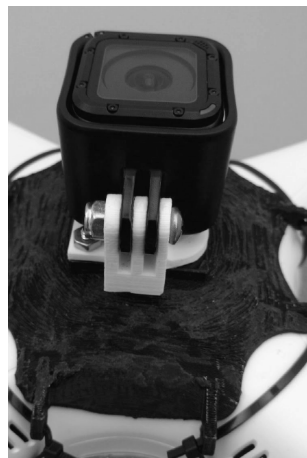
Figure 53: Upward facing optical camera for inspecting the underside of bridge decks
