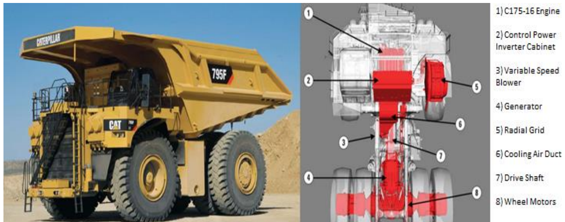
Figure 9: A diesel electric Caterpillar mining truck [19].
