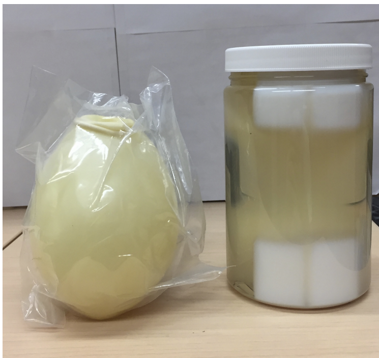
Figure 3.1: An image of a 1 L non-deformable gel dosimeter that's been irradiated next to a 650 mL deformable gel dosimeter in a latex balloon vacuum sealed in low-density polyethylene.
