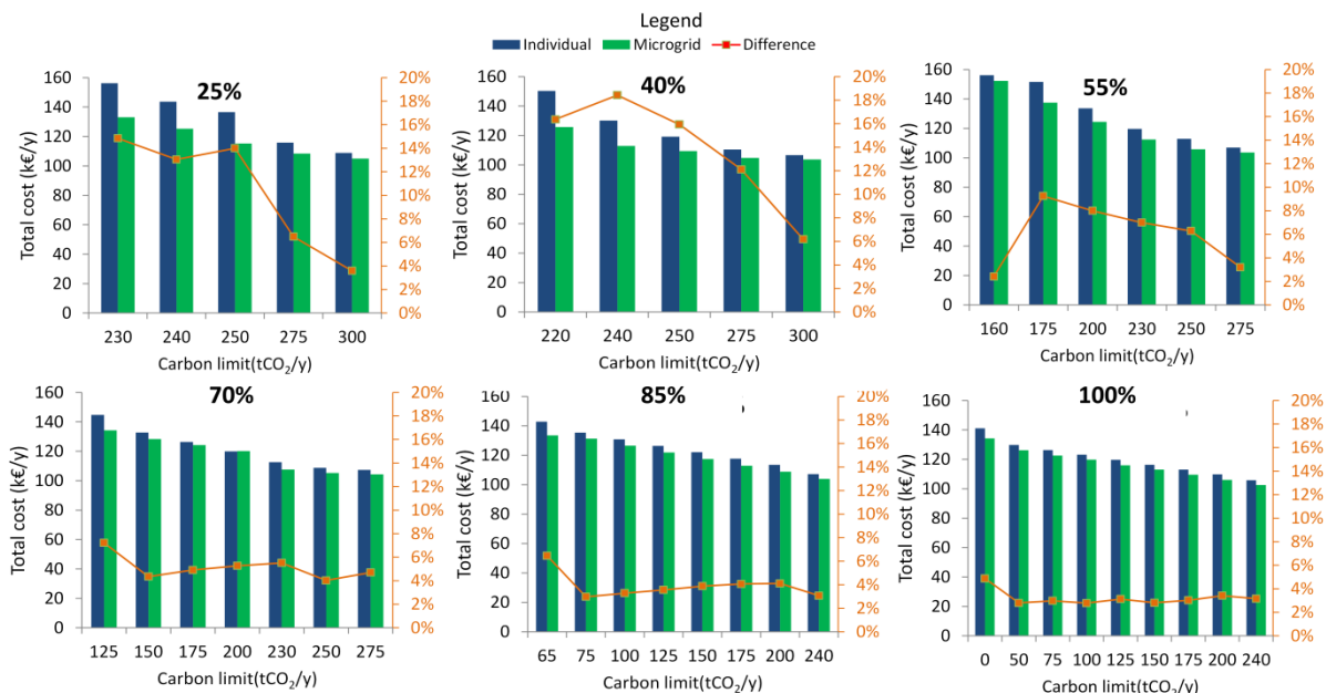
Fig. 2 Total cost for the individual and microgrid approaches for different carbon limits for all scenarios.
