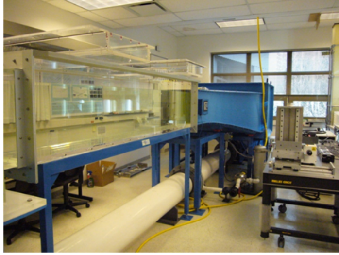
Figure 2.1: Water tunnel used in current experiment.
