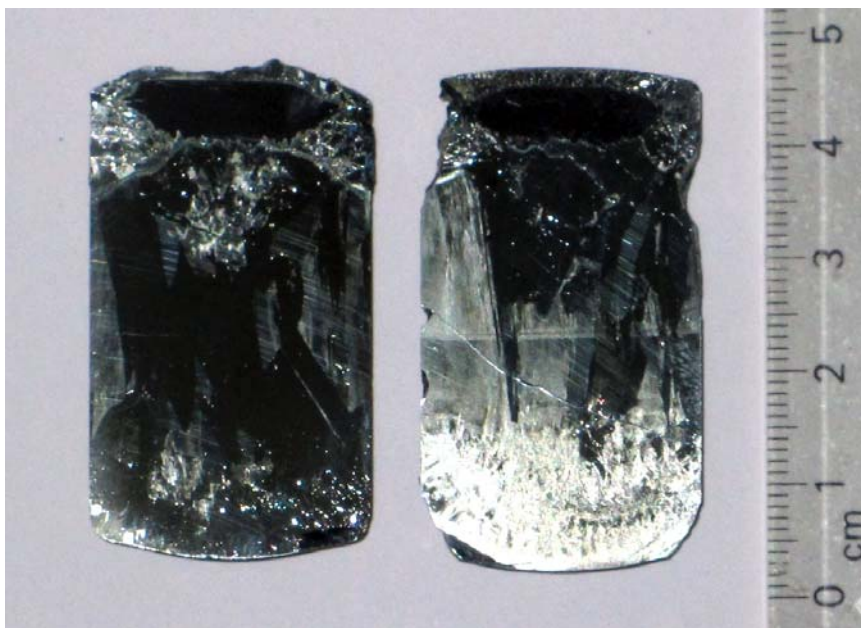
Figure 4.20: The photo above depicts the translated LPD samples. The sample on the left is Translated LPD Experiment #1 and the sample on the right is Translated LPD Experiment #2. In the Translated LPD #2 sample, there is a discontinuity in color visible midway through the sample. This indicates a distinct change in composition. In both samples, large grain structure is visible.
