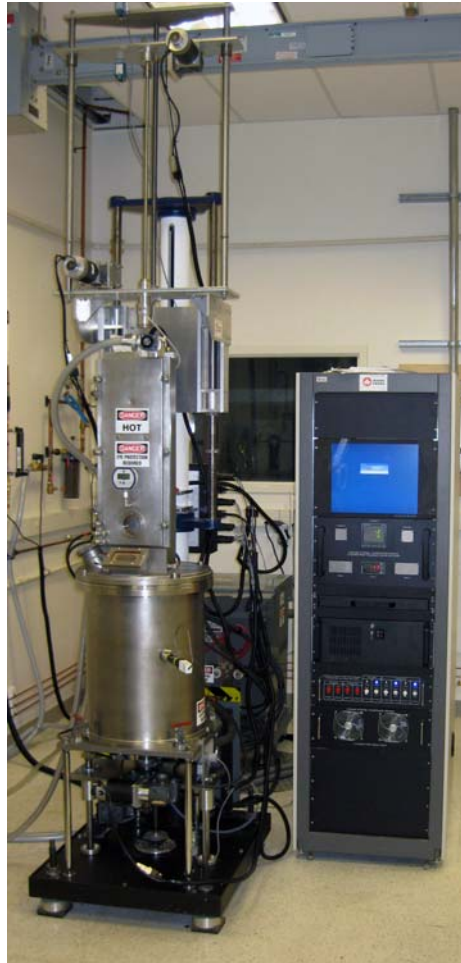
Figure 5.2: The refurbished Czochralski furnace at the University of Victoria is shown above. The furnace has been design and equipped with facilities to allow for the future integration of melt replenishment apparatus.
