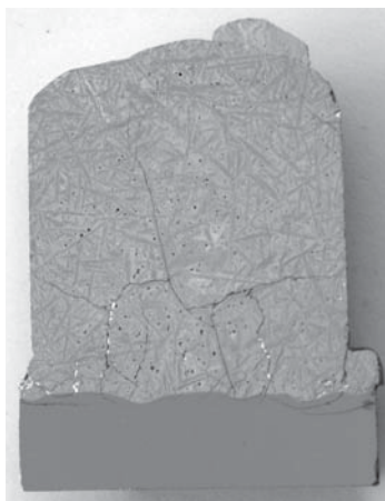
Figure 3.9: The needle structure indicating the presence of silicon is visible in the photo above. A uniform random distribution of the needle structure is apparent.
