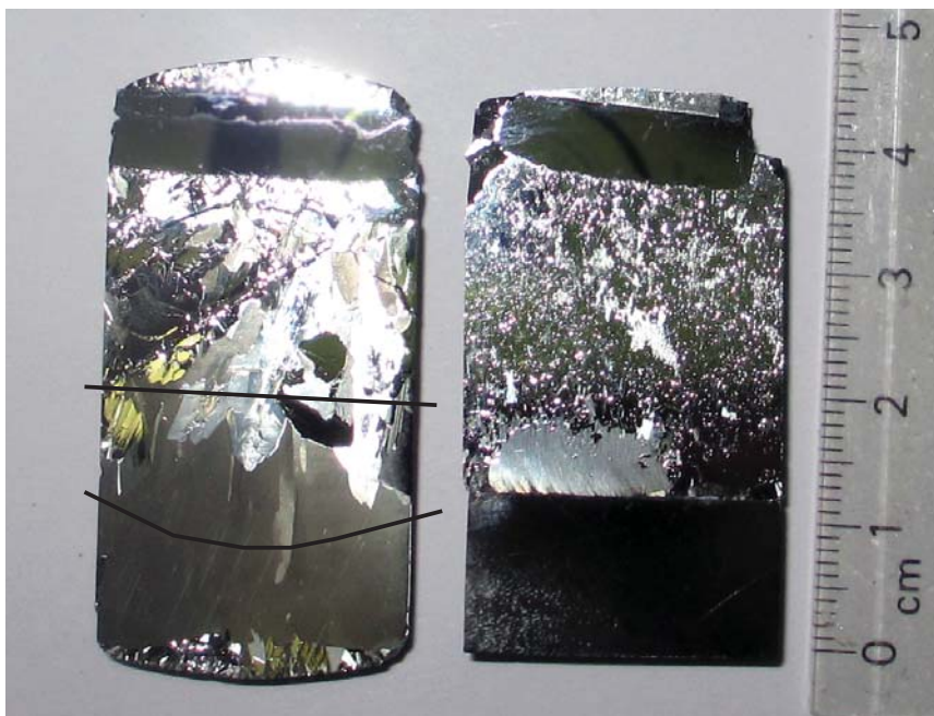
Figure 4.6: The photo above shows the samples processed with the static magnetic field applied. The sample on the left is the Static Field Experiment #1 and the sample on the right is the Static Field Experiment #2. In the Static Field Experiment #2 sample, there was no melt back of the seed and the melt did not fully wet the germanium seed. In Static Field Experiment #1, the seed did wet and there was minor melt back of the seed. The initial growth interface and the limit of silicon in the melt is indicated on the sample by the dark lines overlaid.
