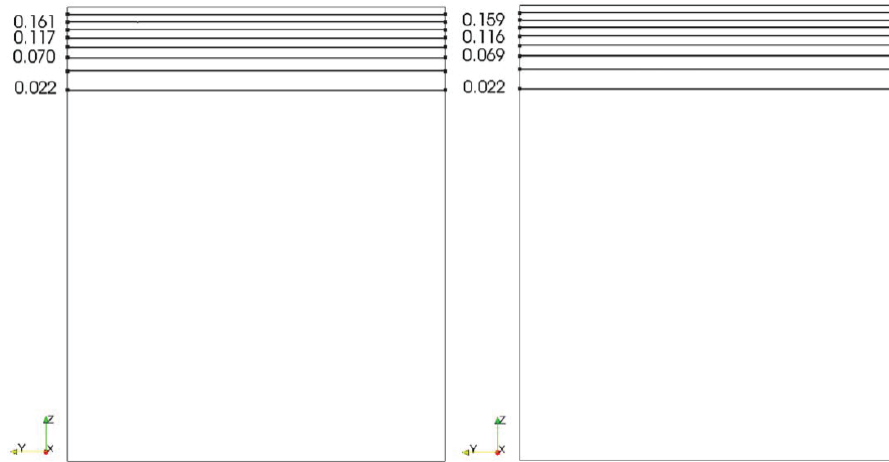
Figure 3.32: The concentration isolines are plotted for two systems without applied magnetic field. The plot on the left is the model with the solutal expansion coefficient set at 5.3 \times 10^{-3} . The plot on the right is the model with the solutal expansion coefficient set at 1.7 \times 10^{-3} . The plots are virtually identical.
