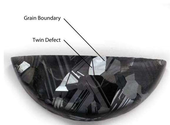
Figure 2.7: The above is a section of polycrystalline CdTe. The grains differ in colouring and have irregular boundaries. Twin defects can be seen in the individual grains. The twins differ from the grain bulk in color and show a very regular boundary through the grain. This boundary will be along a crystal plane. The above sample has been etched to highlight the contrast between grains and twins. Even without the etching, the grains are visible as the reflectivity of the material changes with orientation.
