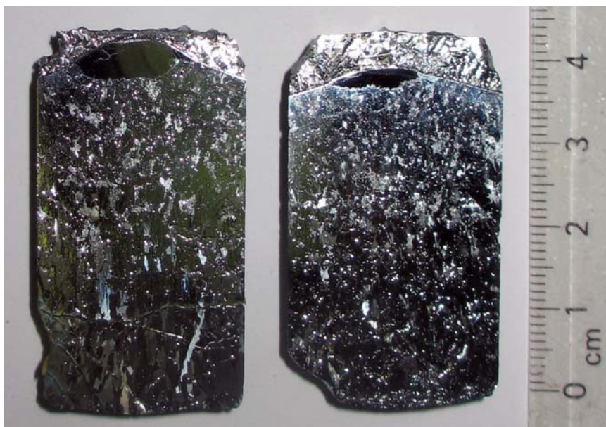
Figure 4.14: The samples above were processed with both the static magnetic field and the rotating magnetic field applied. The seed completely melted back resulting in growth starting with the material self-seeding around the crucible bottom. This has resulted in the material being highly polycrystalline.
