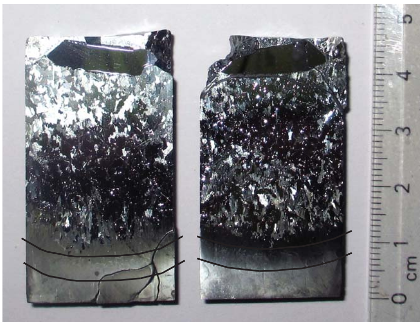
Figure 4.3: The photo above shows the differentially etched sections of the baseline experiment samples. Baseline Experiment #1 is on the left and Baseline Experiment #2 is on the right. The initial growth interface and the extent of single crystal growth is indicated on the photos as dark lines.
