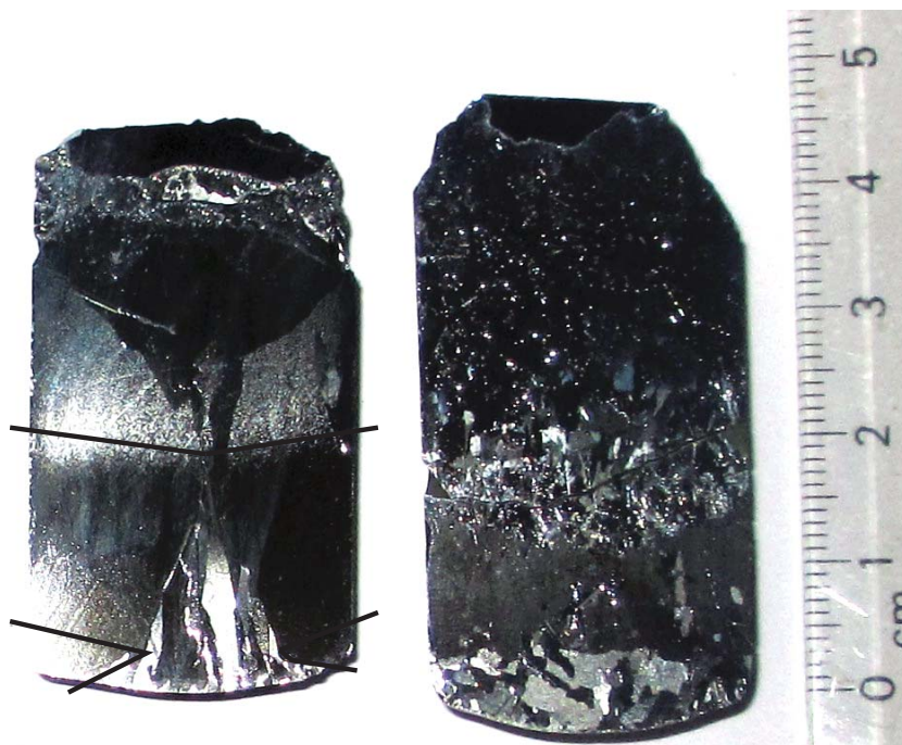
Figure 4.11: The samples processed with the rotating magnetic field are shown above. The sample on the left is Rotating Field Experiment #1 and on the right is the Rotating Field Experiment #2. In the Rotating Field Sample #2, the seed completely melted back and has made the growth material highly polycrystalline. In the Rotating Field Experiment #1 sample, the seed did not melt back fully around the edge of the crucible. This resulted in regions of single crystal being produced around the outside of the crucible. The initial growth interface and extent of growth are indicated by dark lines on the photo.
