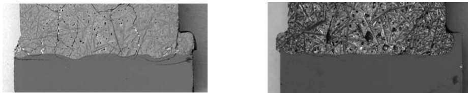
Figure 3.21: The above photos show the dissolution interface shape with and without the applied magnetic field. The sample on the left was processed without the magnetic field. The wavy interface indicating unstable dissolution is evident. The sample on the right was processed with the applied magnetic field. In this case, the dissolution interface is much smoother indicating a more stable process.
