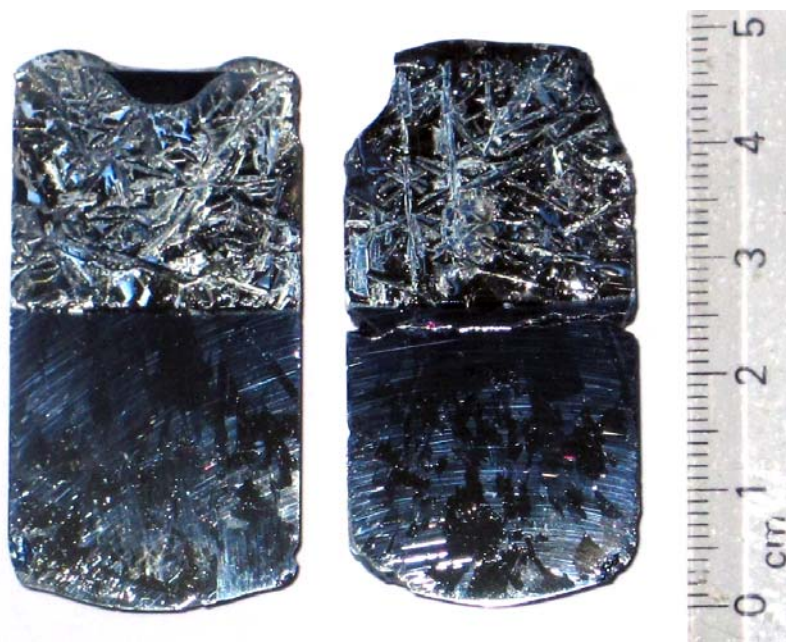
Figure 4.24: The photo above shows the samples processed with the heat sink in place. The discontinuity line midway through the samples is clearly evident. The sample on the left is Heat Sink Experiment #1 and the sample on the right is Heat Sink Experiment #2. The large grain structure of the grown material is visible in the lower area of the samples. The needle structure in the segregated section of the sample is also clearly evident.
