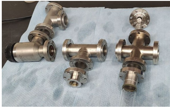
Figure D.4: Air drying the parts after cleaning them
