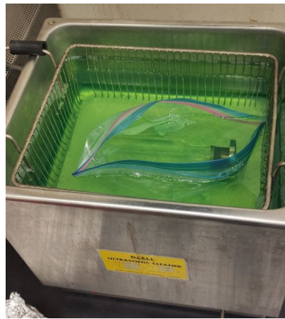
Figure D.5: Ultrasonic bathing parts to get rid of contaminations that are hard to get rid of in a conventional way.
