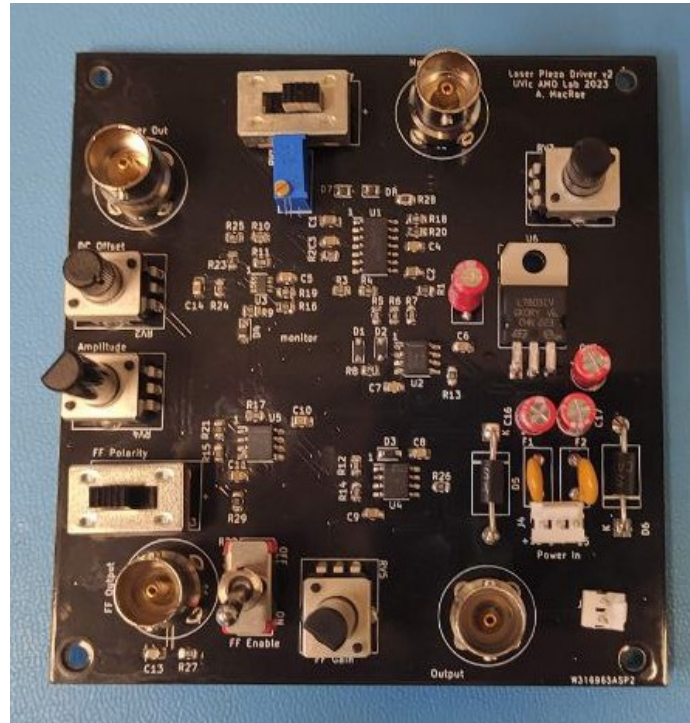
Figure 4.4: Laser Piezo Driver board designed with the help of Andrew MacRae.
