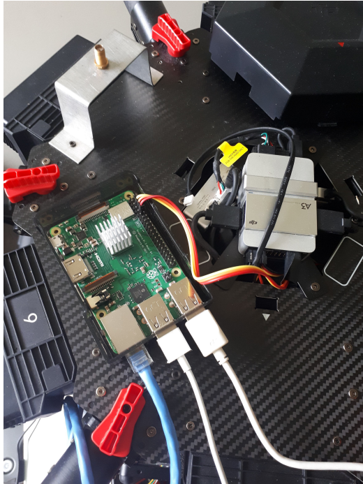
(a) Raspberry Pi connected to DJI A3 by serial connection.
