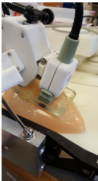
Figure 7.6: Registration of the scanning system with the PBSI template before insertion into an anthropomorphic breast phantom.
