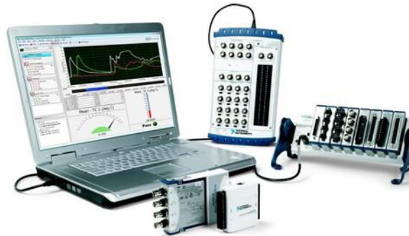
Figure 32 AE Data Acquisitions system
