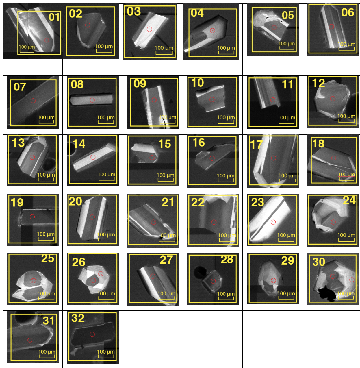
Figure C.3: Cathodoluminescence (CL) images of the zircon grains of samples from Vancouver Island.
