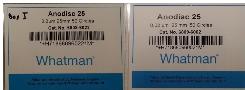
Figure B.1: Anodized Aluminium Oxide membranes purchased from Whatman for this study.
