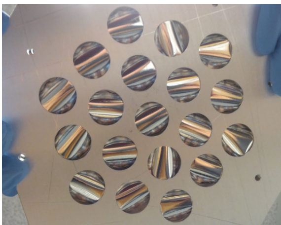
Figure 2.7: Soft and thin polycarbonate templates were curled during the silver contact layer evaporation step.
