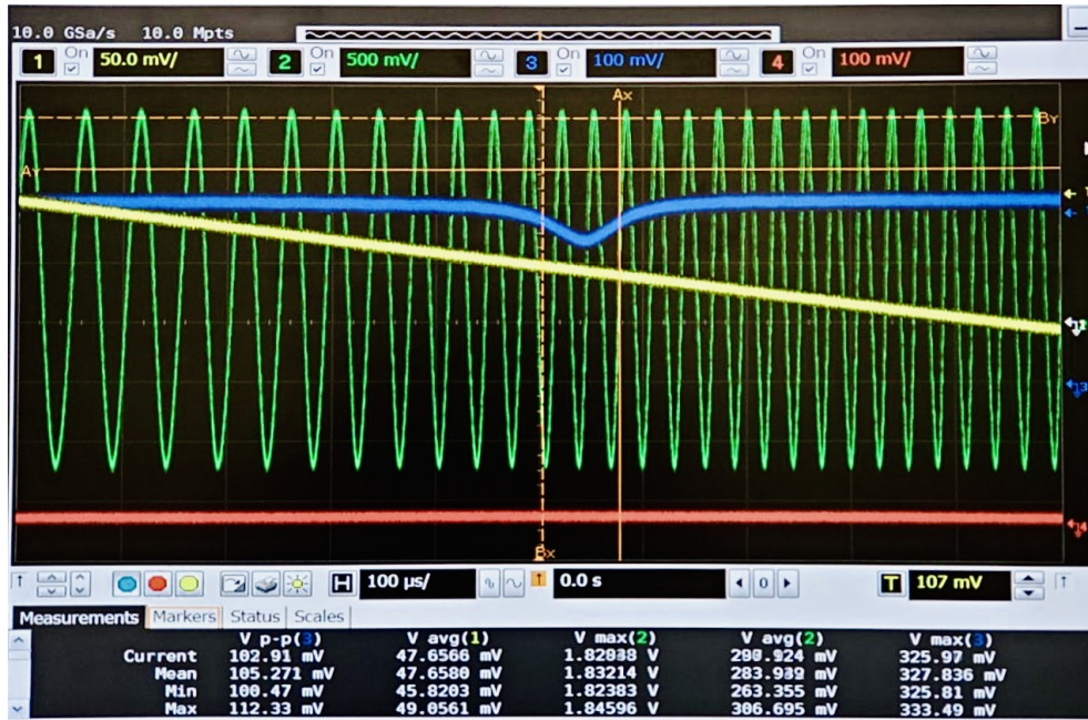
FIGURE 3.20: Lorentzian-shaped signal in the output transmission detected by the tapered fiber shown oscilloscope screen.
