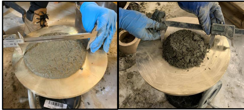
(a) (b) Figure 34. Flow table test a) NC b) P6
