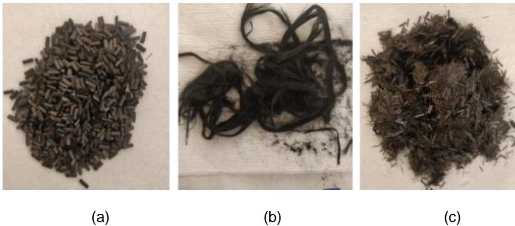
Figure 2. a) pitch-based carbon fibers b) bitumen-based carbon fibers c) PAN-based carbon fibers
