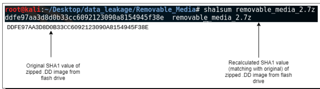
Figure 4.9: Recalculation of checksum from .DD image of flash drive
