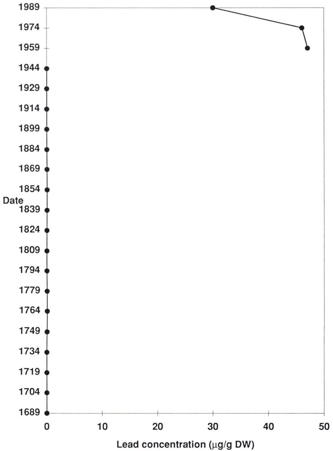
Figure 34. Results of lead analysis performed on north basin core sectioned at 2 cm intervals. Concentrations before 1944 (6 cm) were not detectable.
