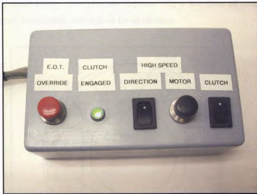
Figure 31 Controller for Linear Translator
