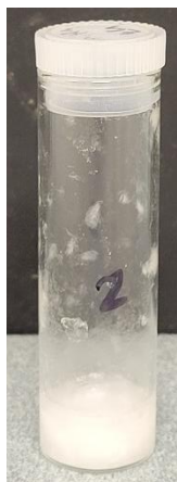
Figure S5.7: Image of 1 (0.8% w/v), 5mM CB[6] and 100 mM NaCl in 20% aqueous EG, 1 week after gelation experiment.
