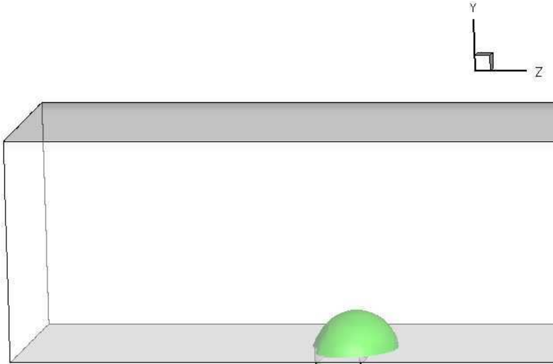
Figure 53: Phase boundary dynamic contact angle, 1cm/s water injection, 4m/s air speed at a time of 2ms, water droplet emerging from a pore
