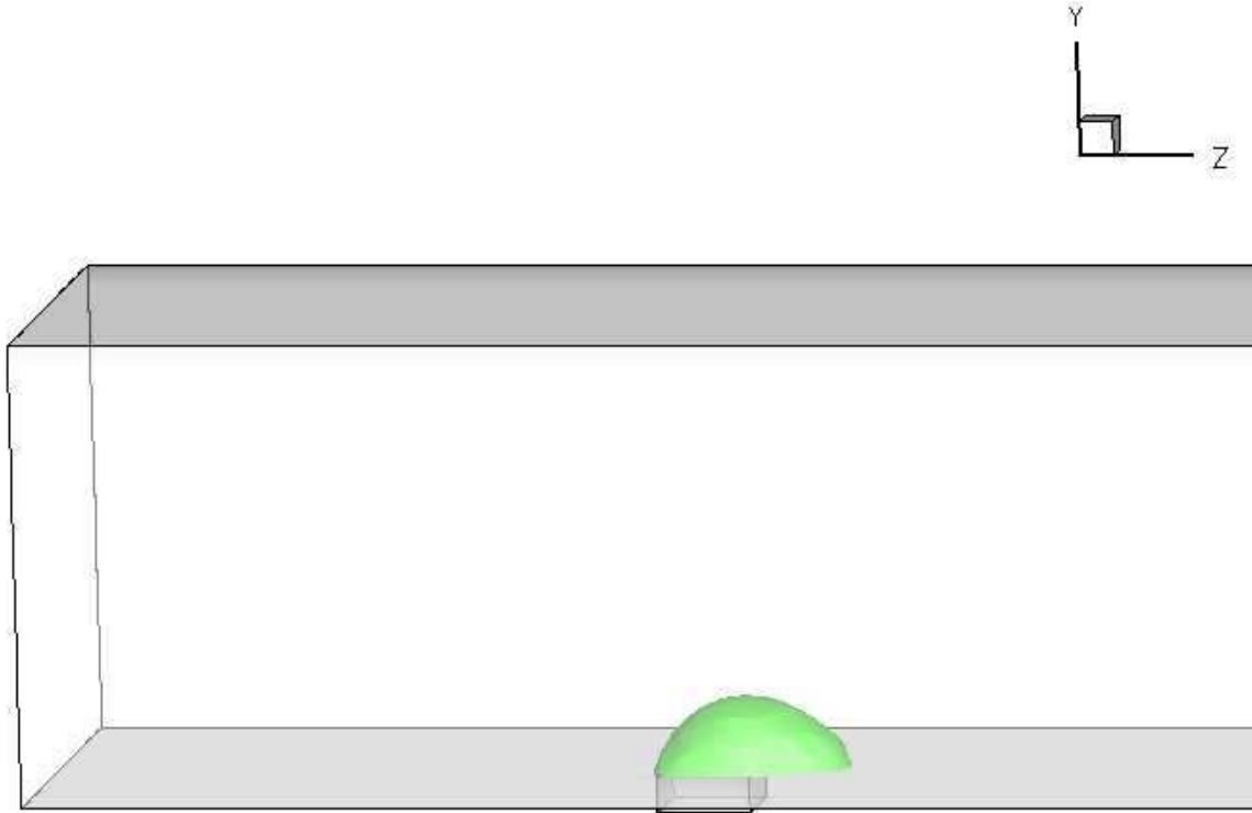
Figure 66: Phase boundary, 2cm/s water injection, 10m/s air speed at a time of 2ms, water droplet emerging from a pore
