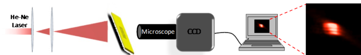
Figure 3. Schematics of the experimental setup used for SPR imaging acquisition.
