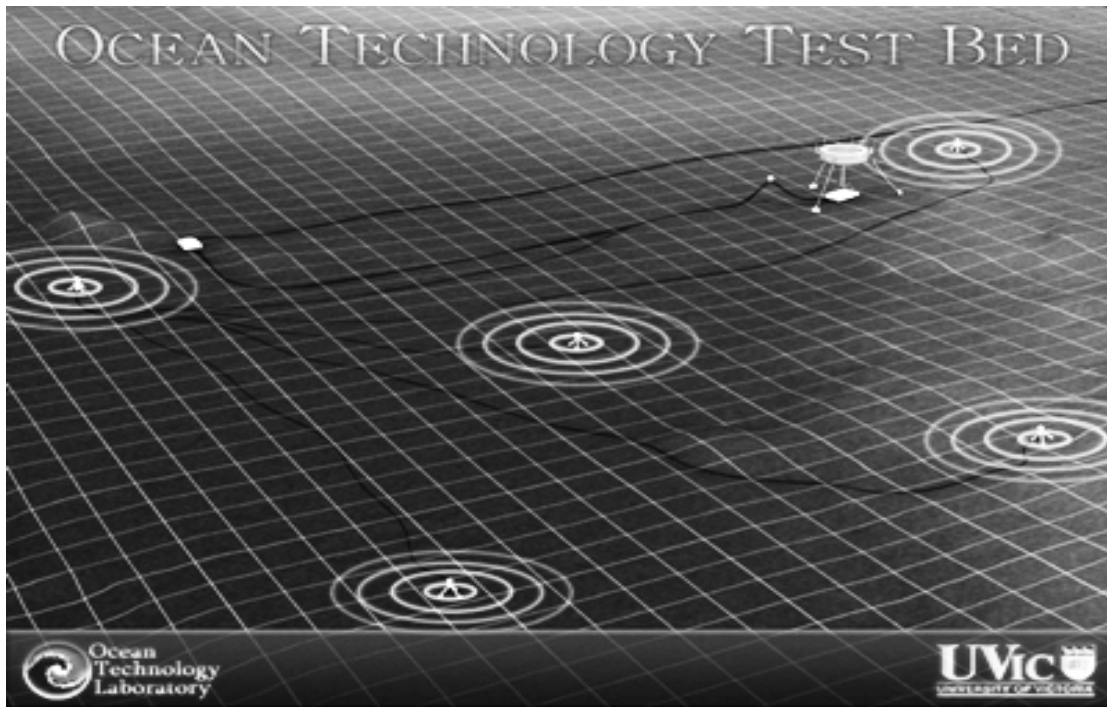
Figure 1.2: Conceptualized layout of the University of Victoria's Ocean Technology Test Bed infrastructure. Concentric circles indicate location of five cabled receiver towers (Ocean Technology Lab, 2005).
