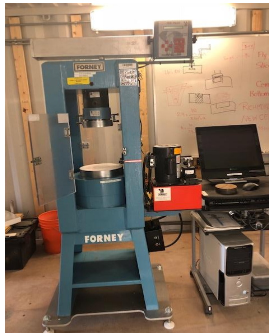
Figure 6 Forney's Compressive Strength Test Machine
