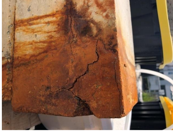
Figure 15 OPC beam after 200 hours of test
