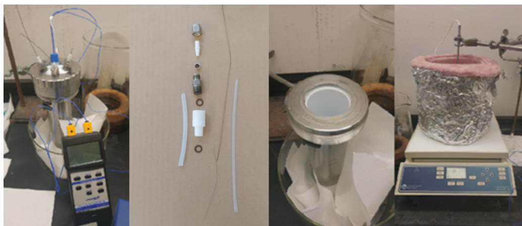
Figure 2.2: Autoclave setup. The self-pressurizing autoclave setup used for high temperature electrochemical experiments. The first panel shows the assembled autoclave with the digital temperature probe used for calibrating the internal temperature. The second panel shows the electrode assembly. Heat-shrink teflon tubing is used to allow only a small portion of the nickel wire to be exposed to solution. The remainder of the assembly prevents any steel pieces from being exposed to solution, while also keeping the autoclave pressurized. The third panel shows the cell interior, a teflon sleeve of single piece construction. The fourth panel shows the ramping hotplate with an insulated beaker on top. The beaker is filled with silicone oil and a temperature probe is placed inside.
