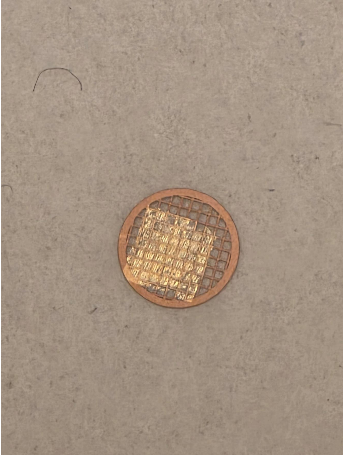
Figure A4. A 200-mesh copper grid bearing an ultrathin section. A 200-mesh copper grid bearing an ultrathin section collected from the water trough of the diamond knife, ready for TEM examination.
