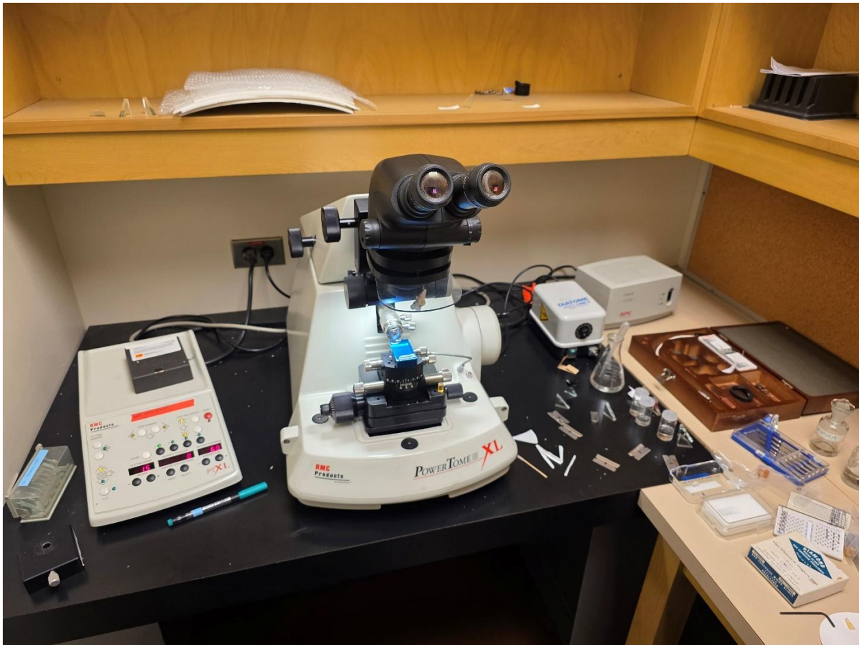
Figure A1. RMC PowerTome XL ultramicrotome. An RMC PowerTome XL ultramicrotome used for cutting semithin and ultrathin sections from resin-embedded tissue blocks. A diamond knife is visible mounted in the ultramicrotome.
