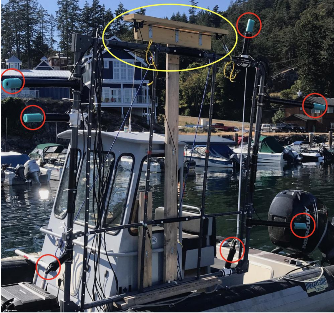
Figure 3.5: Hydrophone array configuration for 2020. Red circles show the new positioning of the M36 Geospectrum hydrophones. Yellow circle shows the newly installed pulley system. The Reson hydrophones had not been installed at the time of this photo.
