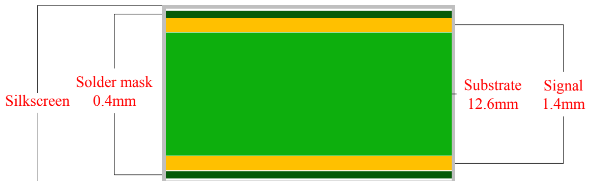
Figure 3.13: Layer structure of the designed double-sided PCB.
