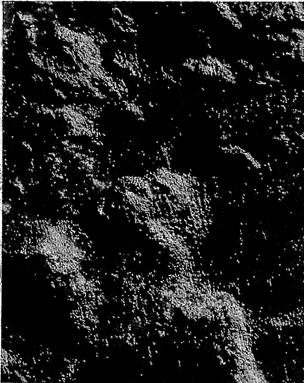
Figure 4.7. Bathymetric image of multibeam data set D2 that was cleaned using the automatic outlier detection method.
